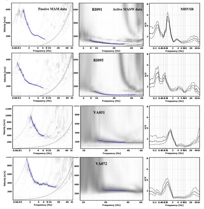
Fig. 2 Input parameters for inversion at the 4 considered sites. (Left) Dispersion estimates from passive-source MAM data with picked dispersion curve in blue. (Middle) Dispersion estimates from active-source MASW data with picked dispersion curve in blue. (Right) Average +/- one standard deviation MHVSR curve from all sensors in the smallest and largest arrays.
