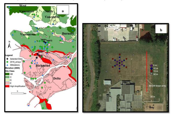
Fig. 1a: Location of array measurements conducted in July 2018 (green crosses) and co-located with strong motion stations (blue triangles) in Metro Vancouver. Site Class microzonation map is modified from [15]. 1b: Geometry of passive circular arrays and MASW linear array location at Site RI095.
