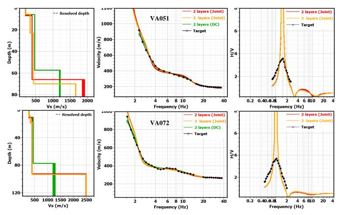
Figure 3: Shear wave velocity profiles obtained with different model parameterizations for the 4 selected sites (left), the theoretical and experimental phase velocity dispersion curves (middle), and theoretical ellipticity function with experimental MHVSR peaks (left). Joint refers to joint inversion results and DC refers to dispersion inversion only.
